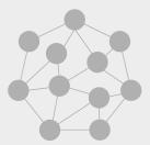
Wireless mesh network - network topology characterized by the absence of a central node through which the entire communication takes place. Instead, each node in the network acts as a transmitter of data to other nodes.
